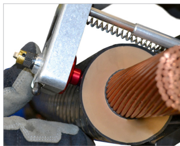
Easily clamp onto the cable width, adjusting for various cable sizes.
