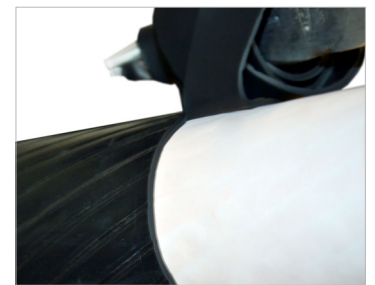
Square off the continuous chip with a clean, burr-free radial cut.
