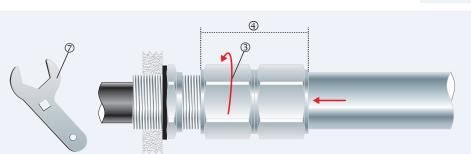
4 Pass the cable end through the conduit assembly 3 and the gland assembly. Tighten the outer 3 to the installation torque using a CCG Spanner 0 to produce a seal and grip on the cable.
