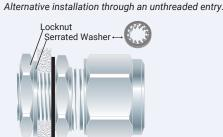
If the apparatus is untapped use a locknut.
