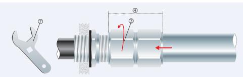
Pass the cable end through the conduit assembly ④ and the gland assembly. Tighten the outer ③ to the installation torque using a CCG Spanner ⑦ to produce a seal and grip on the cable.
