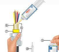
6. Re-insert the barrier pot sub-assembly 6 back into the inner 2.
