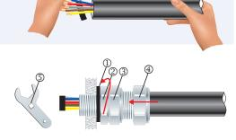
Unscrew the coupling nut ③. Withdraw the cable and barrier pot sub-assembly ⑥. Remove the insulation tape.
