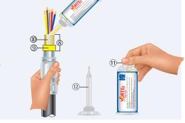
Re-insert the barrier pot sub-assembly 8 back into the inner 2.
