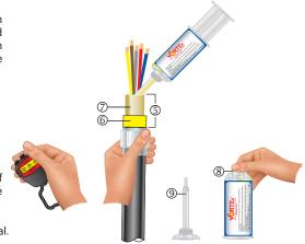
6. Re-insert the barrier pot sub-assembly 5 back into the inner 2.
