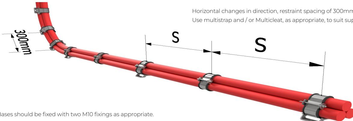
Horizontal changes in direction, restraint spacing of 300mm maximum.
