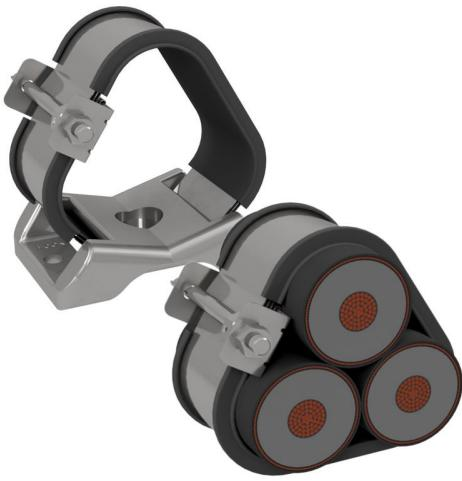
Multicleat and multistrap now use a new and improved locking mechanism making the installation quicker and easier. They also come with a disposable tensioning aid that was introduced in response to customer requests to improve the closure of the cleats and speed of installation. The adapter fits into the open end of the winding pin and is used with a standard 13mm socket wrench to tighten the strap. The same 13mm socket is then used to tighten the locking nut, finishing the installation.
