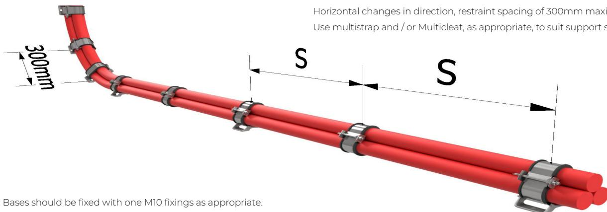
Note: Bases should be fixed with one M10 fixings as appropriate.
