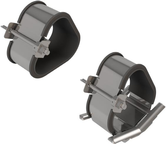
Multicleat and multistrap now use a new and improved locking mechanism making the installation quicker and easier. They also come with a disposable tensioning aid that was introduced in response to customer requests to improve the closure of the cleats and speed of installation. The adapter fits into the open end of the winding pin and is used with a standard 13mm socket wrench to tighten the strap. The same 13mm socket is then used to tighten the locking nut, finishing the installation.
