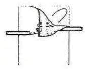
1. Wrap connector with Scotch 27 or 69 Class Cloth Tape. Position bottom of connector in center of pad. Fold corner over connector. *Stretch* pad around the cable
