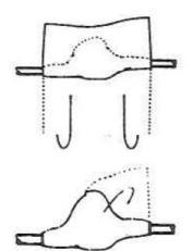
3. Fold bottom of pad up over connector.
