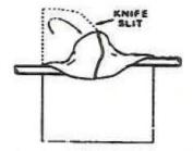
2. Make knife slit and fold other corner over the top of the connector. *Stretch* pad around the connector.
