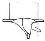
2. Fold other corner over connector. *Stretch* pad around cable and connector.
