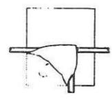
1. Wrap connector with Scotch 27 or 69 Glass Cloth Tape. Position connector in center of pad. Fold left corner of pad over connector. *Stretch* pad around cable and connector.
